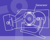
Some hand powered flashlights have a capacitor that stores short bursts of energy. If your flashlight has a switch it has this type of storage and you may need to add another step on your energy diagram.
