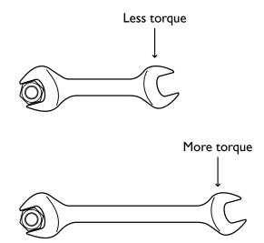
On a commercial wind turbine, the long blades of the turbine generate lot of torque to the generator. Utility-scale wind turbines often have large gearboxes that increase the RPM of the rotor by 80 or 100 times. This big gear reduction demands a lot of torque from the blades. Think about riding your bicycle— when you shift into a higher gear, it may be harder to pedal. A higher gear ratio demands more force which generates more torque.
