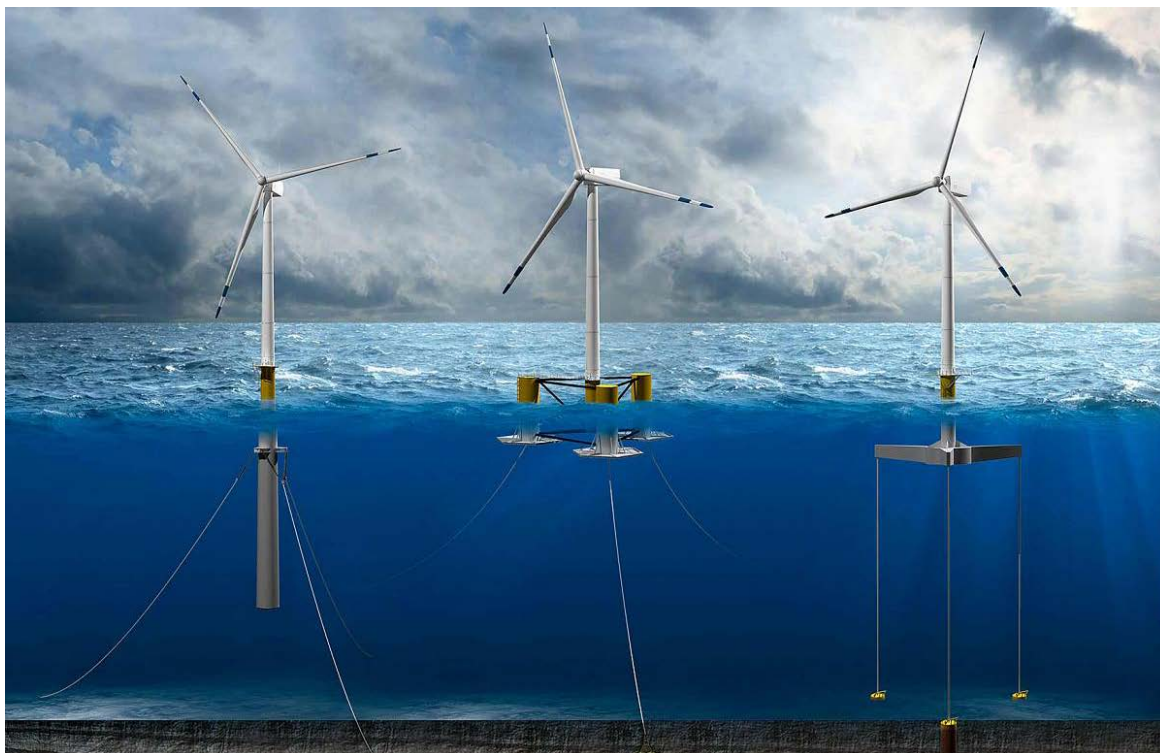
Visual representation of the different ways to design floating offshore wind turbines.
